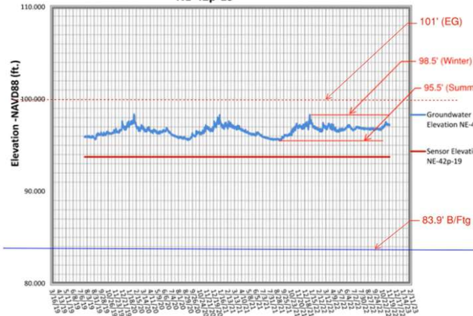
Figure C-24. Groundwater Elevation Versus Time NE-42p-19
